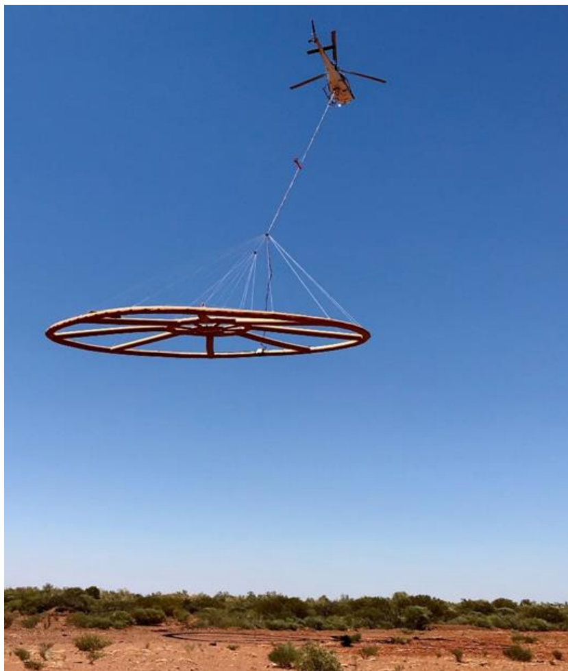
Figure 2 AEM Survey Helicopter in action
