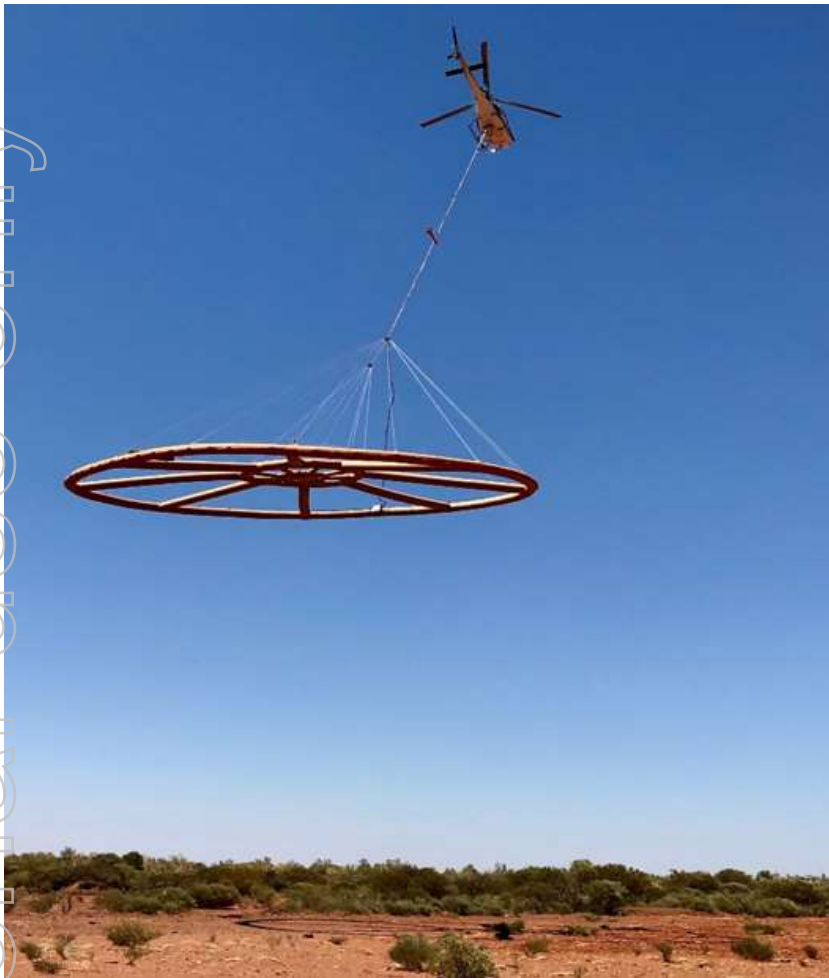
Figure 3: AEM Survey Helicopter in action
