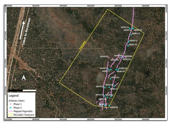
Figure 1: Mt Deans RC drilling along the interpreted pegmatite
