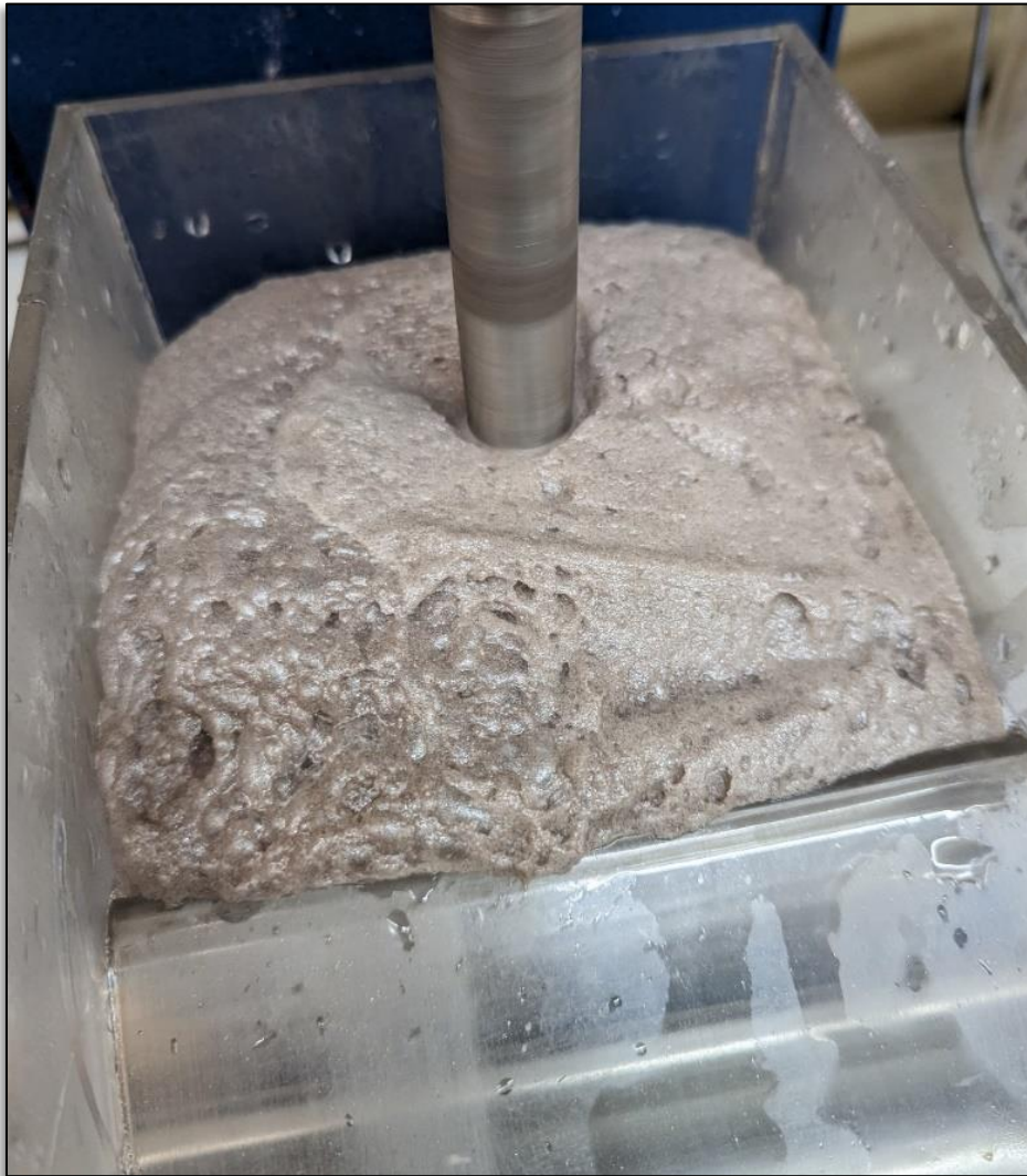
Figure 4: Mt Deans sample undergoing flotation test.
