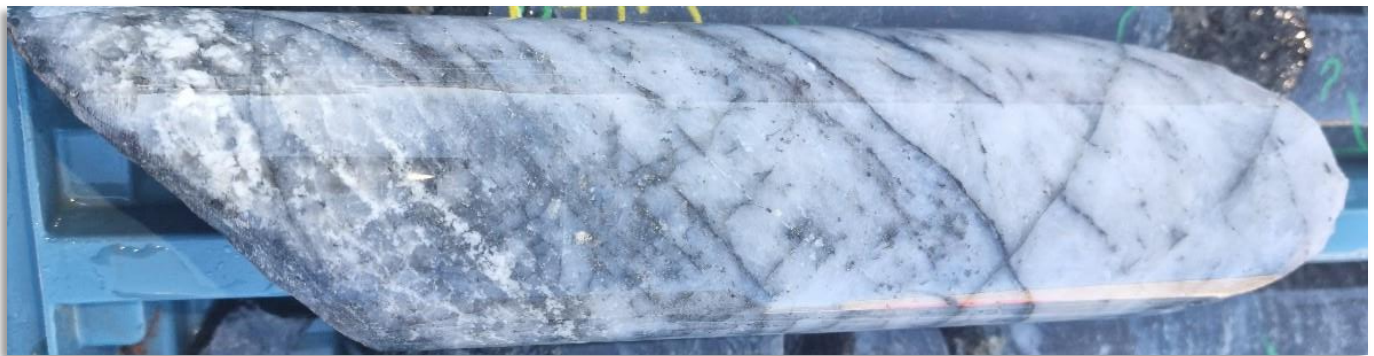
Figure 3. Drill core from SG23DD003 from 43.4m to 43.6m showing Norseman style quartz lode mineralisation with disseminated sulphide.
