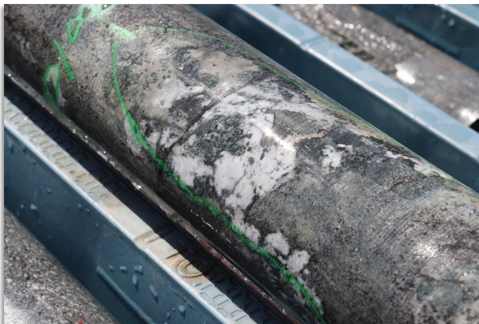
Figure 4. Drill core from SG23DD009 from 54.3m to 54.5m showing disseminated sulphide associated with the quartz lode mineralisation.
