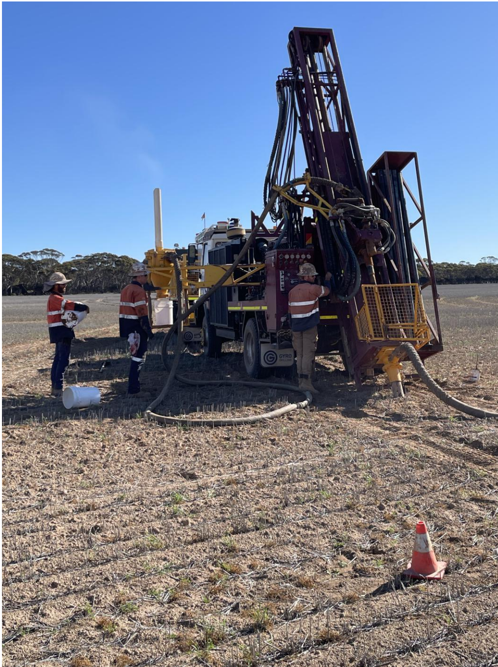
Figure 11: Salmon Gums Aircore Drilling, April 2025
