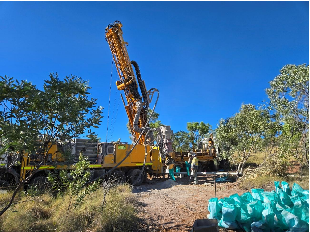
Figure 4: Aruma's RC drilling at the Piper Prospect, Fiery Creek project
