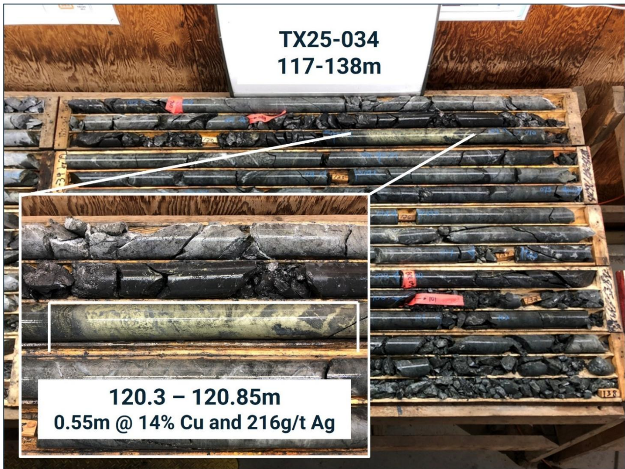
Figure 5: Diamond Drill Core showing high-grade massive chalcopyrite intersection from drill-hole TX25-034
