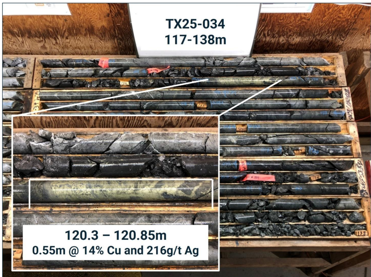
Figure 5: Diamond Drill Core showing high-grade massive chalcopryite intersection from drill-hole TX25-034
