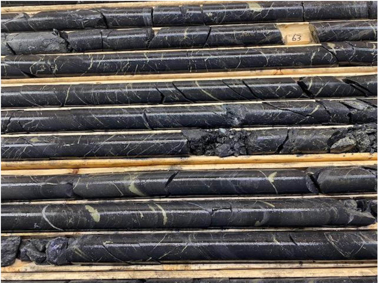
Figure 3: Diamond Drill Core showing high-grade chalcopyrite intersection from drill-hole (TX25-034); 98.2m @ 1.82%Cu and 13.17g/t Ag from 35.8m
