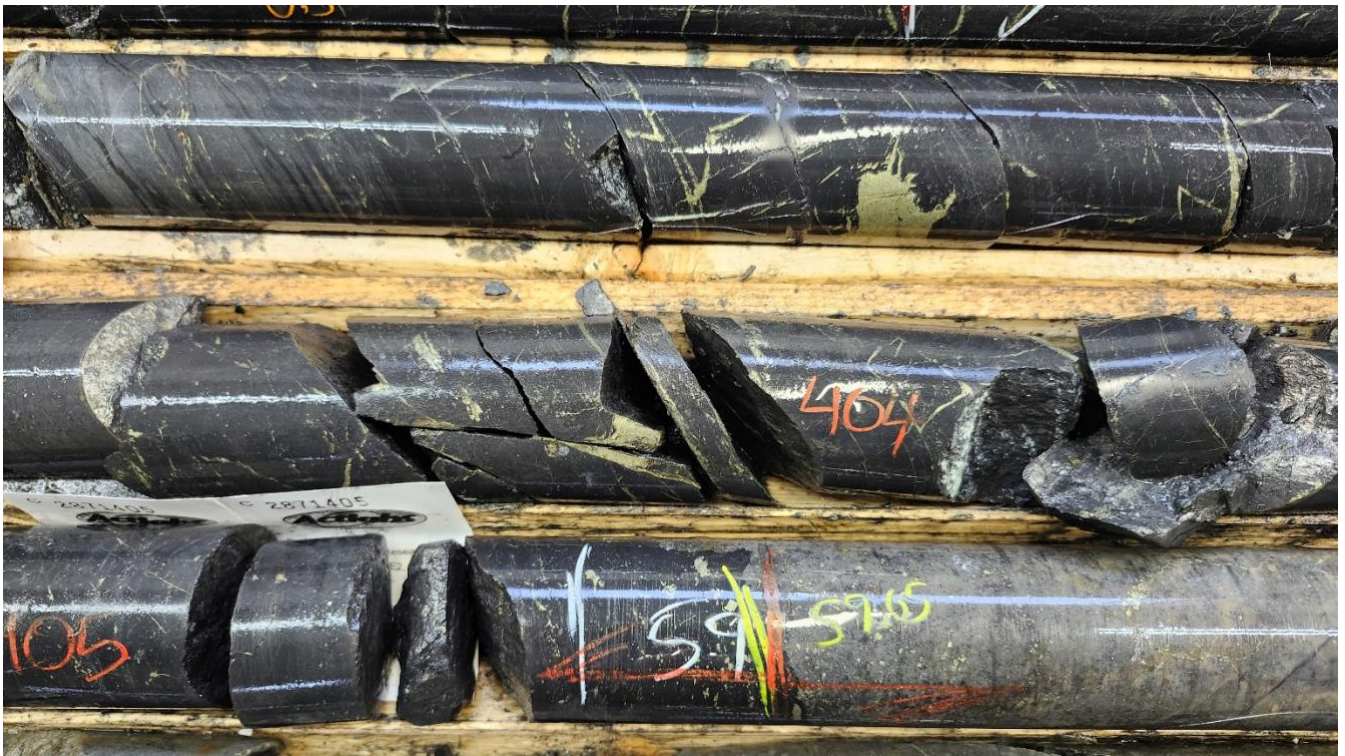
Photograph 2: Tillex Project TX26-005 Diamond Drilling Core, Mineralised Porphyry/Argillite Contact @59m Depth
