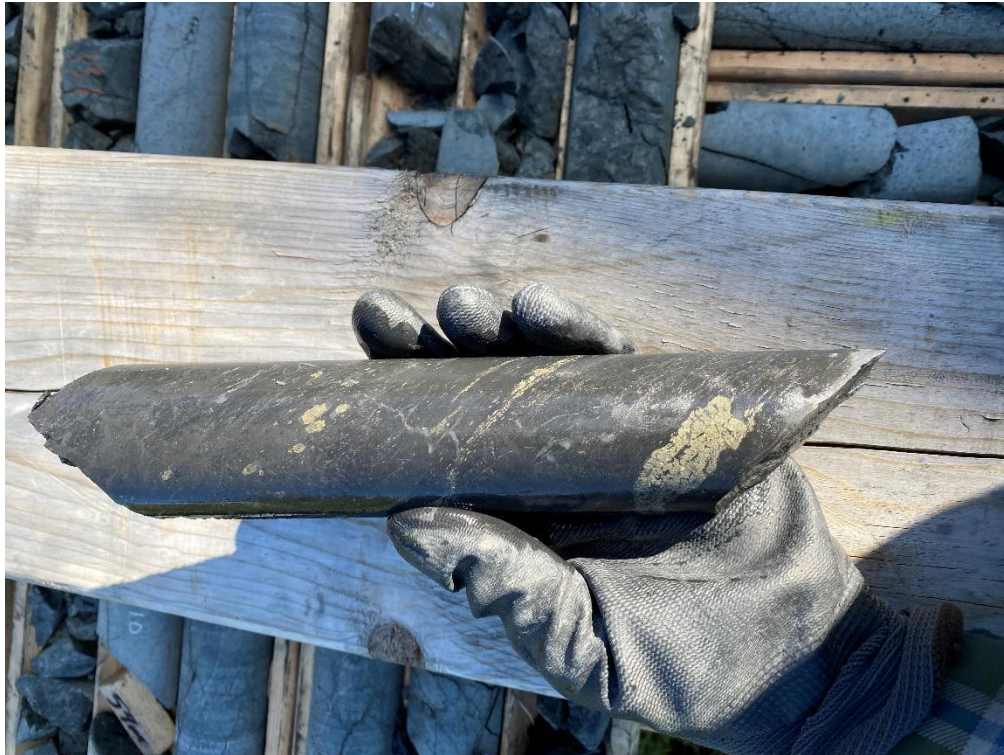
Photograph 3: Tillex Project TX26-007 drill core at 184.9m, disseminated, fracture fill and coarse chalcopryite within argillite – assays returned 3m @ 0.45% Cu and 3.3g/t Ag from 182m
