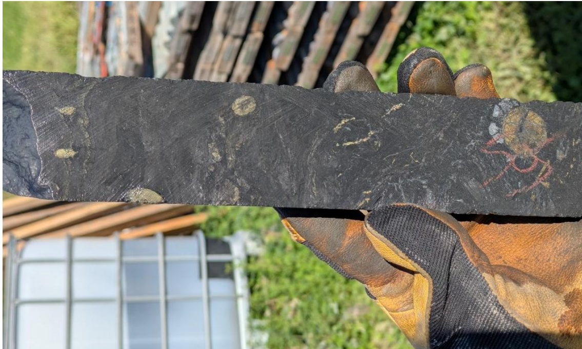
Photograph 2: Tillex Project TX26-006 drill core at 95m, disseminated and coarse chalcopryite with minor quartz carbonate veining within argillite – assays returned 14m @ 1.38% Cu and 5.0g/t Ag from 83m
