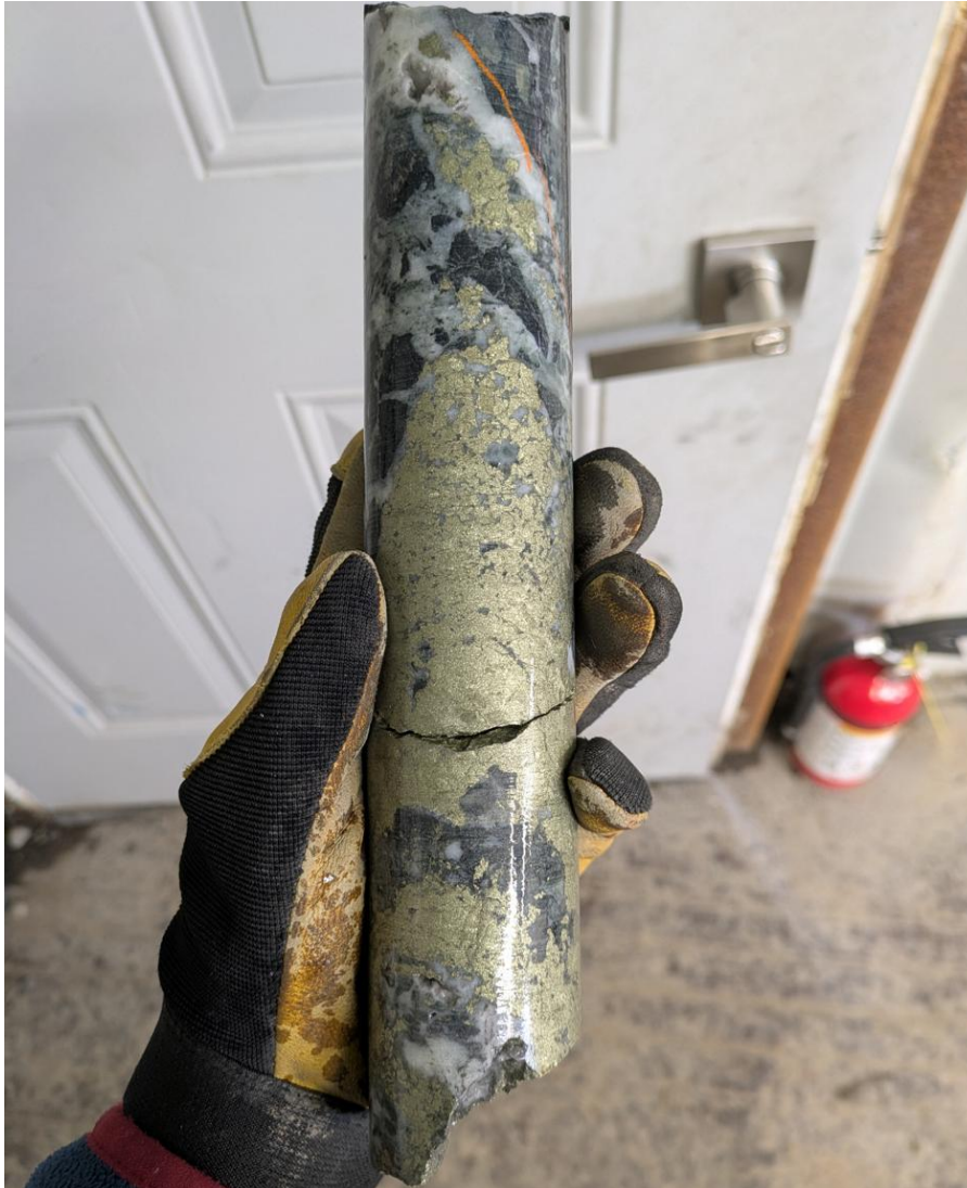
Figure 3: TX26-012 drill core semi massive chalcopyrite and pyrite within a fault breccia; 0.34m @ 15.5% Cu and 110 g/t Ag from 114.44m.
